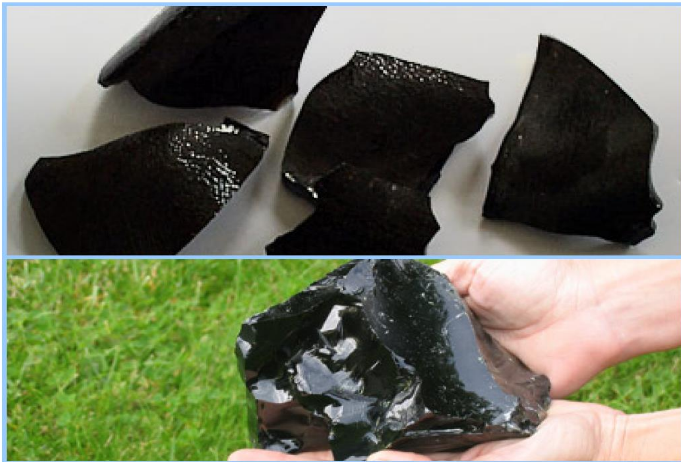
Diagram 32: Vitrified, glass-like, inert slag
